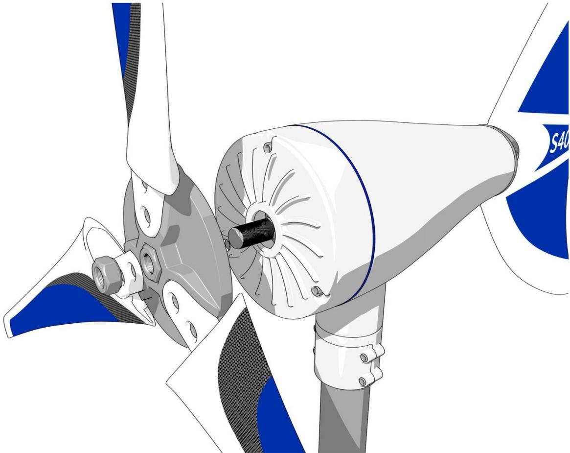
Attention: During this work on the rotor it must be ensured that the rotor cannot start. The 3 wired cable must be short-circuited. Otherwise, the rotor can start running and cause injuries.
