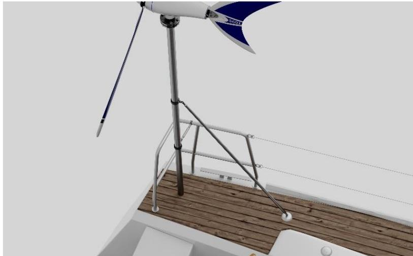
Note: Please note that the SHARKY S401 can never achieve its full performance if it is not in the main wind direction or is deflected. Therefore, it is important to find a suitable location that is free of obstacles in the prevailing wind direction!
