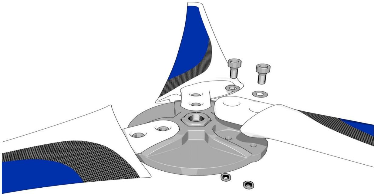
The blades are balanced by the shape of the hub disc by the special type of manufacture (conical mount).
